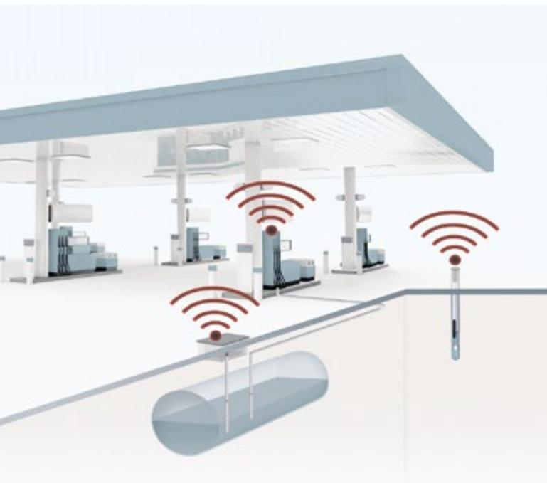
Graphical example of monitoring and leak detection at a service station.
